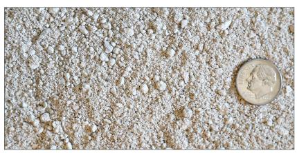
**ABOVE**: Compost Sugar has a 1/8-inch top-end stone size with extensive fines content. **RIGHT**: Compost Sugar is layered into the compost feedstock, providing a buffer to the volatilization taking place in the decomposing matter, mitigating nitrogen loss, and providing inert bulk that improves airflow. Then, once in the soil, pumice provides long-term soil performance improvement on a structural level, long after the compost is consumed.
