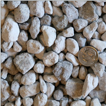
LEFT: Ponics Stone Standard contains stones from 3/4-inches to 5/16-inches in size. RIGHT: Ponics Standard used as the grow media in a flood-and-drain aquaponics grow bed.
