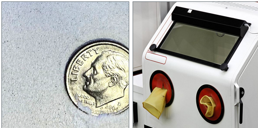
LEFT: Sand Blast Fine (SBF) grade pumice blast media. RIGHT: SBF is a fine-grained, gently-aggressive blast media used for delicate and/or detailed surfaces.
