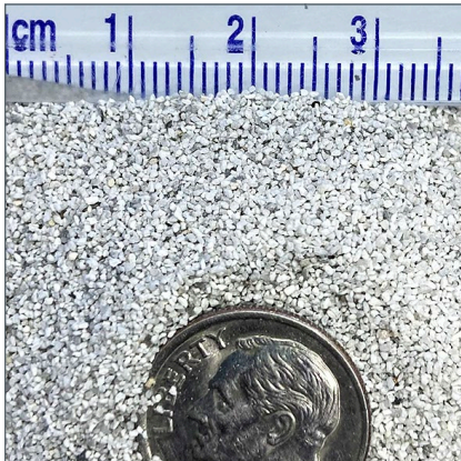
LEFT: Sand Blast Soft (SBS) grade pumice blast media. RIGHT: SBS is a smaller sand blasting grade for cleaning more delicate surfaces.
