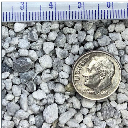
LEFT: Sand Blast Standard (SBH) grade pumice blast media includes approximately two percent “heavy” igneous minerals, which are not removed through our mining processes. RIGHT: Sand Blast Standard being used as a blast gun media.
