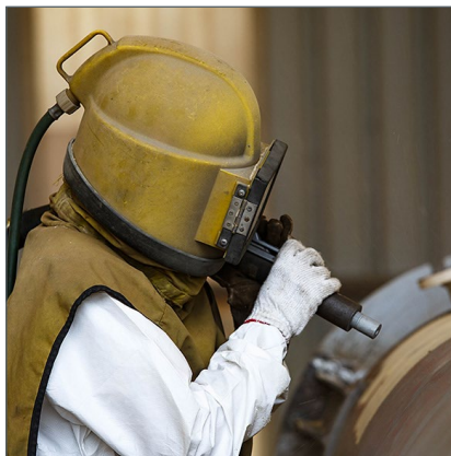
LEFT: Sand Blast Standard (SBH) grade pumice blast media includes approximately two percent “heavy” igneous minerals, which are not removed through our mining processes. RIGHT: Sand Blast Standard being used as a blast gun media.
