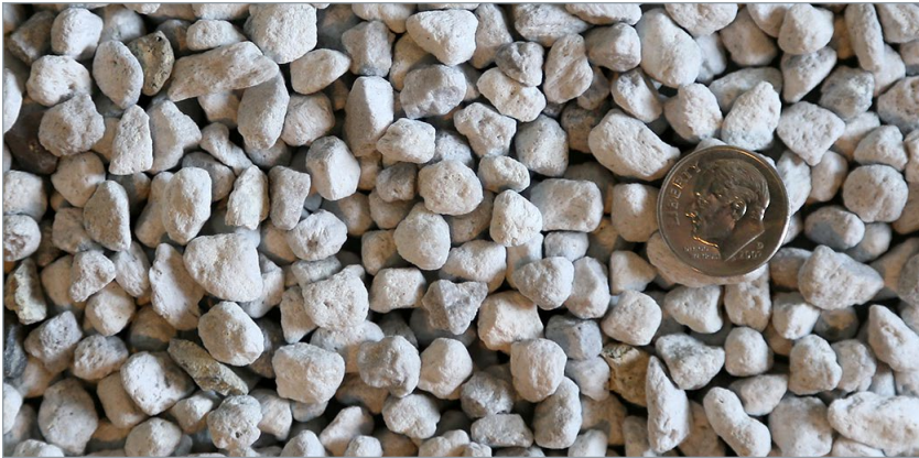
SoilRox Mulcher C is primarily 5/16-inch stones with no fines.
