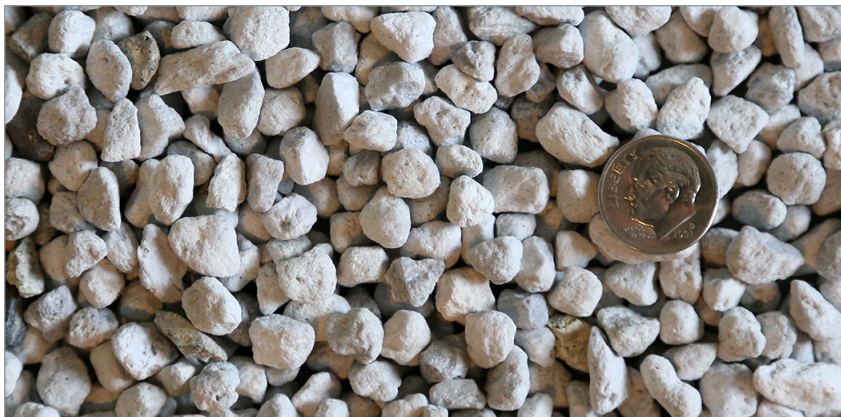
HP Grade five-sixteenth inch stones dried, cleaned, and free of fines.
